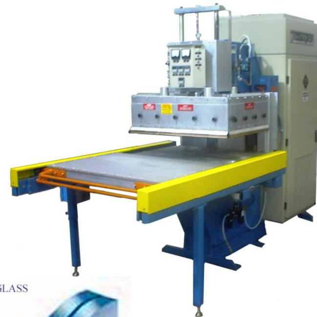
Thermex Thematron RF Press with shuttle
