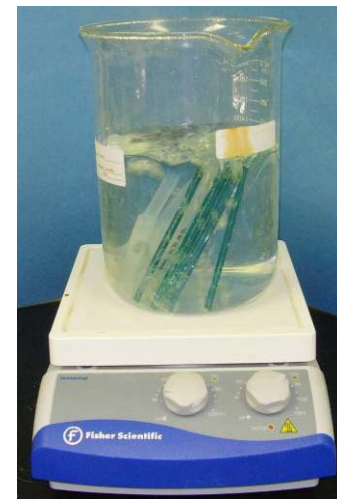
Boil Testing RF Laminated TPU
