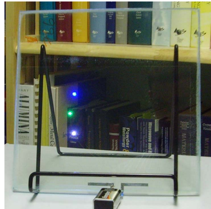
3-color LED after press Blue-Green-White (top to bottom) 9" square glass with PVB
