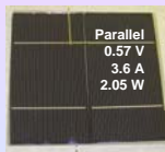
Dual cell solar panel Wired in parallel 6" x 6.5" glass with PVB
